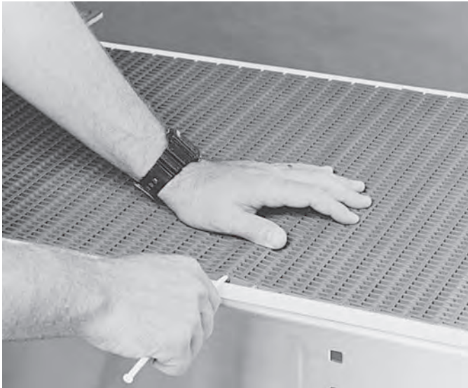
Figure 1: Plastic modules joined by hinge rods
