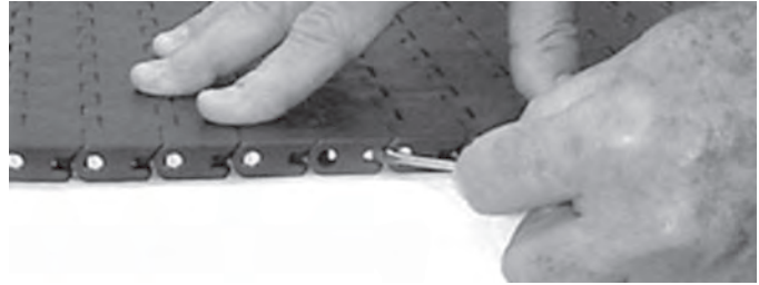
Figure 51: Slidelox rod retention
